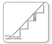
**B.** Tighten the first rail bracket in place so when turned over the back of the bracket touches the rear of the first step from the bottom landing. Place the other rail on the last step before the top landing, again tightening it so it touches the rear of the last step.
